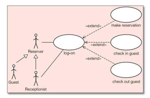
Figure 8 Making log-on the main use case
