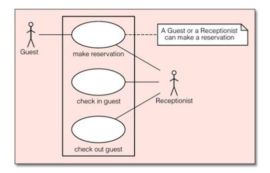
Figure 3 A use case model for a system for checking in and out of a hotel
